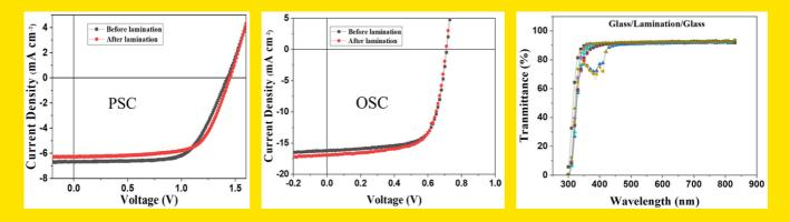
The successful lamination enables our prototype tandem cells to be characterized. These first generation four terminal cells have good PCE in a current matching stacked tandem configuration. The quantum efficiency (EQE) is as expected for the component cells.
