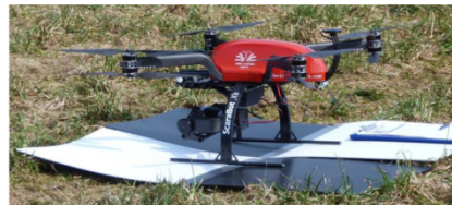
Fig. 1. The remote-controlled octocopter with integrated IR and RGB cameras used for the generation of the aerial IR data.
